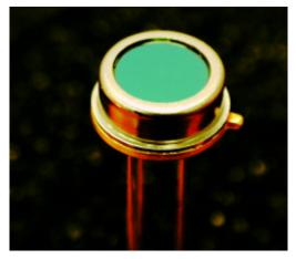
SCD-Si detectors are packaged with a short cap (0.13 inches tall) to maximize the field of view (FOV). Optimizing the FOV is particularly important for applications that monitor a large area such as for gas or fire detection at an oil refinery or large manufacturing plant.
